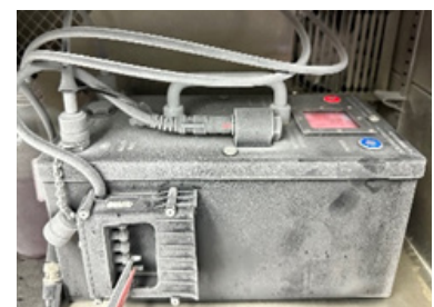
Environmental chamber testing at -30°C
